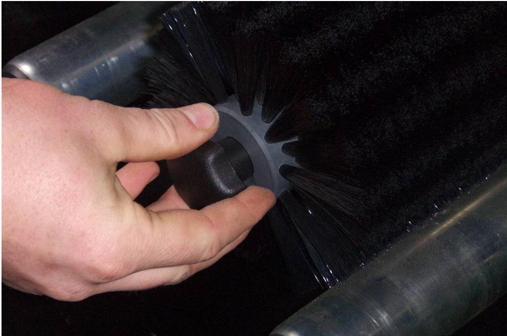
Picture E: The brushes can easily be mounted and demounted by loosen the black thumbscrew.
